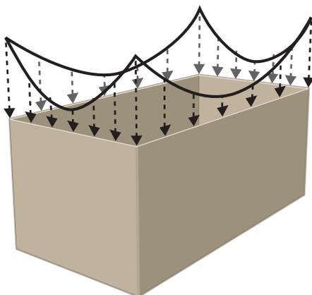
The length of the dotted arrow is proportional to the load bearing ability at that point.
