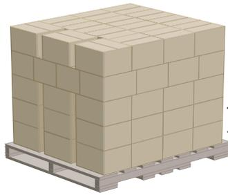
Composed of column lower layers plus an interlocked upper layer.
